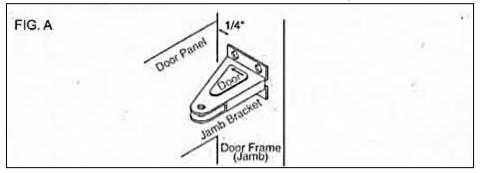
At desired height, fasten jamb bracket to storm door frame with open side ¼" from door as shown. (See Fig. A). If more latching force is desired, jamb bracket may be moved up to 1" away from door.
