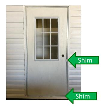
3. <u>Do NOT open the door or remove shipping clips</u> <u>or shims before installation.</u> Opening the door before installation will destroy the proper squaring of the door. If shims are not in place, position one shim at the bottom of the door core butting the striker side frame and underneath the core. Position the other shim near the striker plate between the core and the frame.
